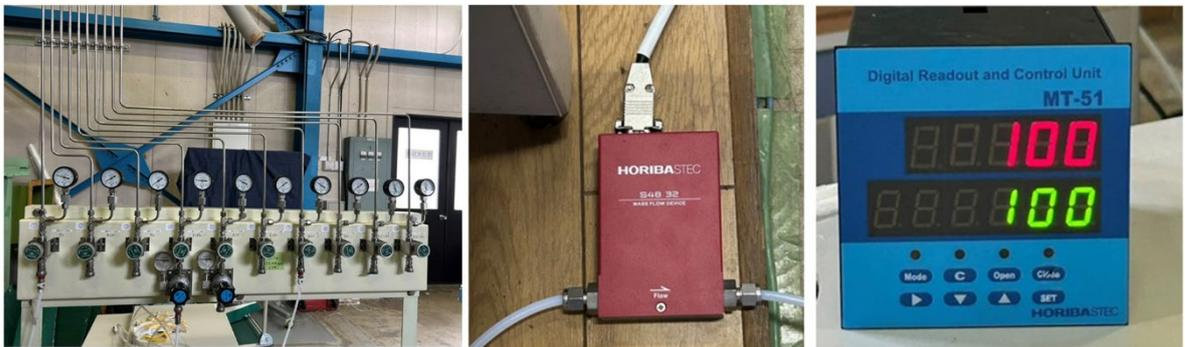
Figure 7. Gas supply station and mass flow controller.
