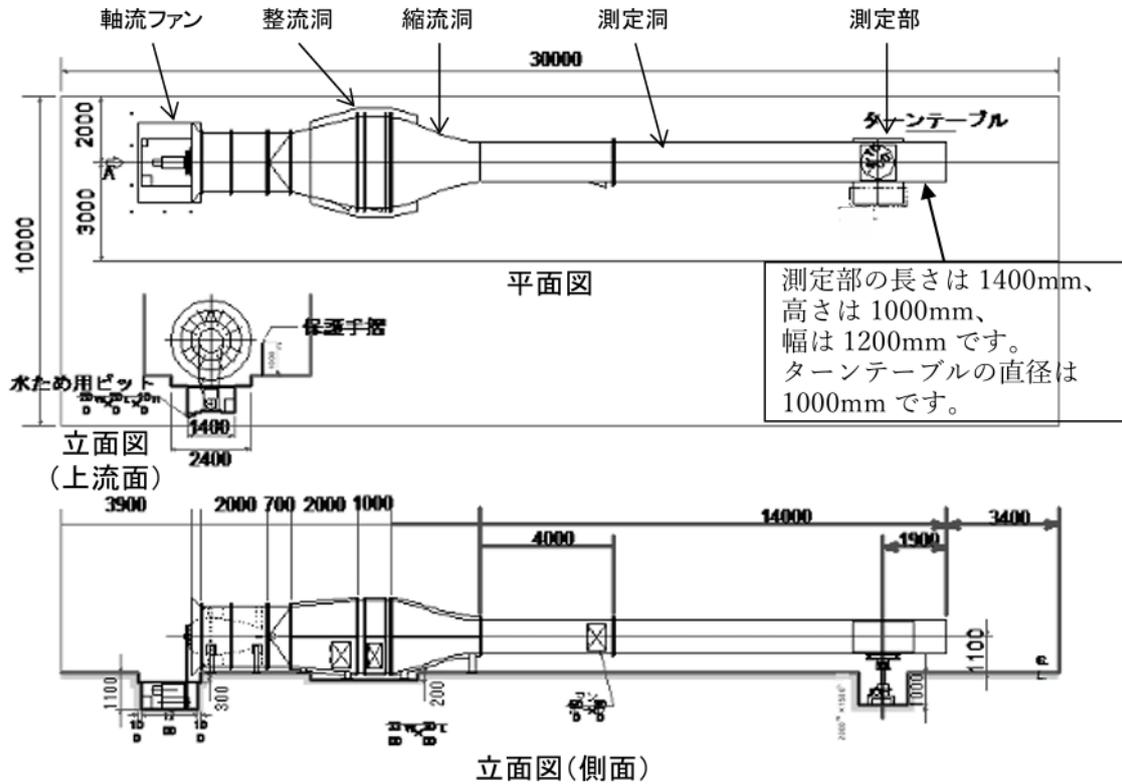
Figure 3. Wind tunnel plan and elevation view.
