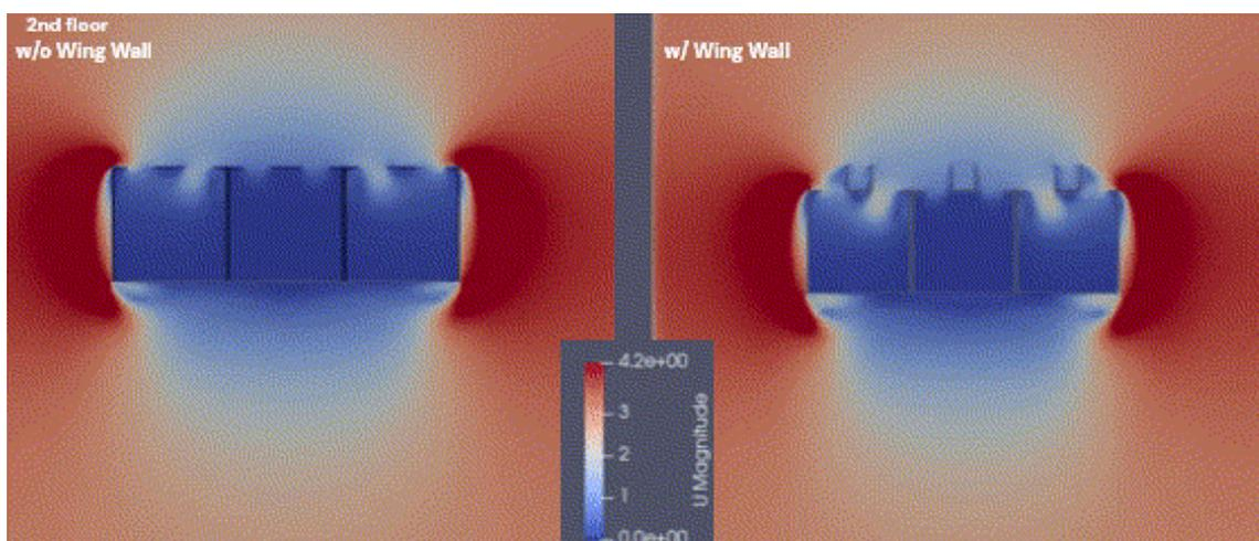
Figure 16. Velocity distribution at the second floor without wing wall (left) and with wing wall (right).
