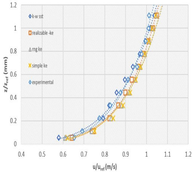
Figure 13. CFD and Wind Tunnel comparison.
