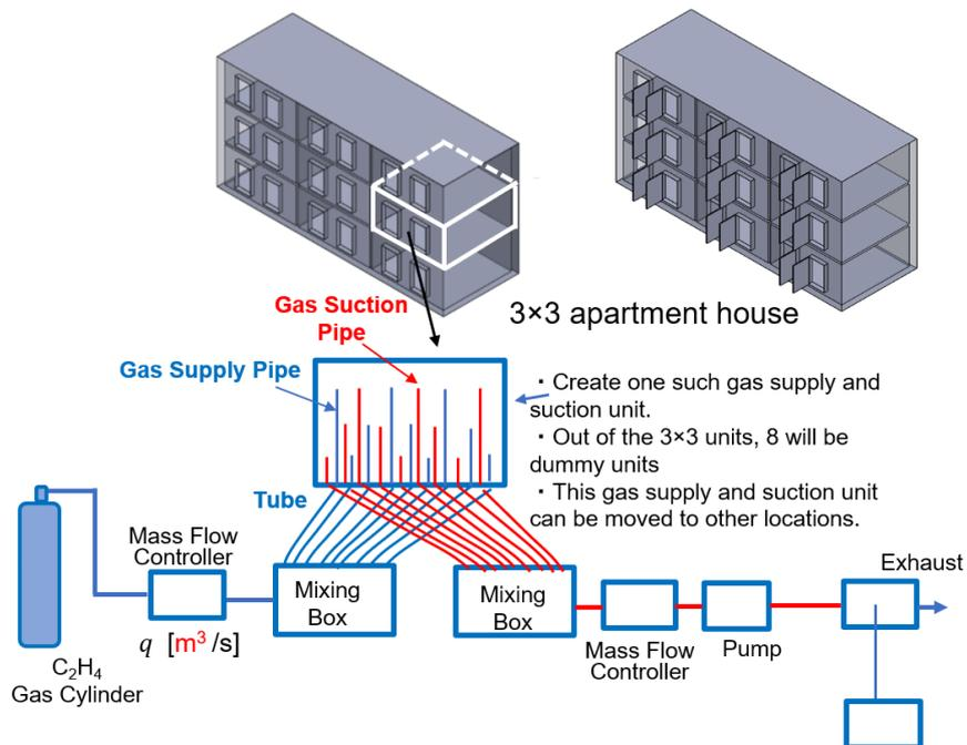
Figure 5. Setup for tracer gas method.
