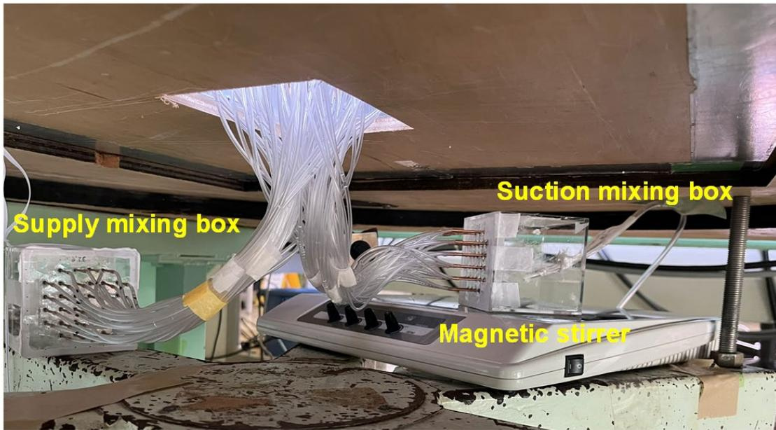
*Figure 8. Installation status of the mixing box under the wind tunnel floor.*
