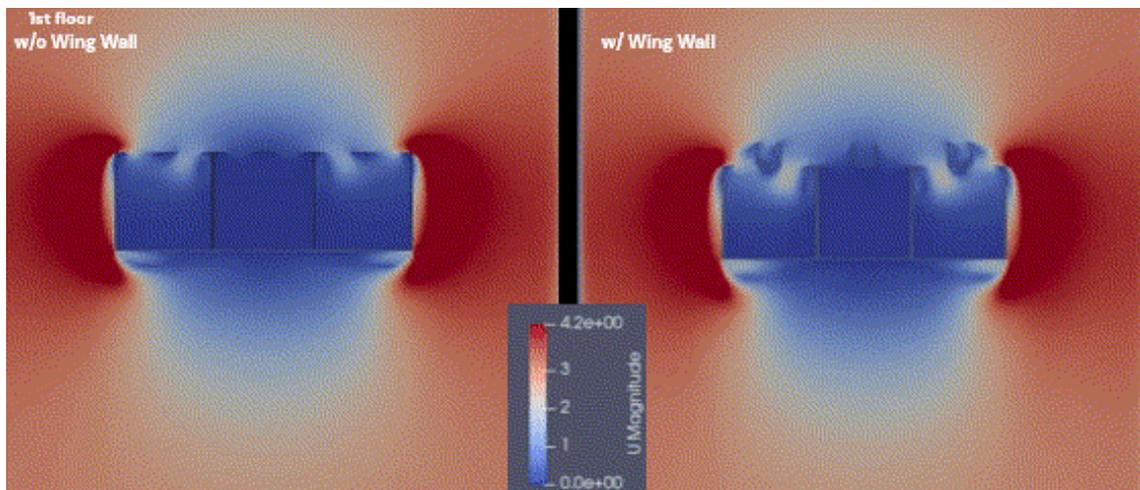
Figure 15. Velocity distribution at the first floor without wing wall (left) and with wing wall (right).
