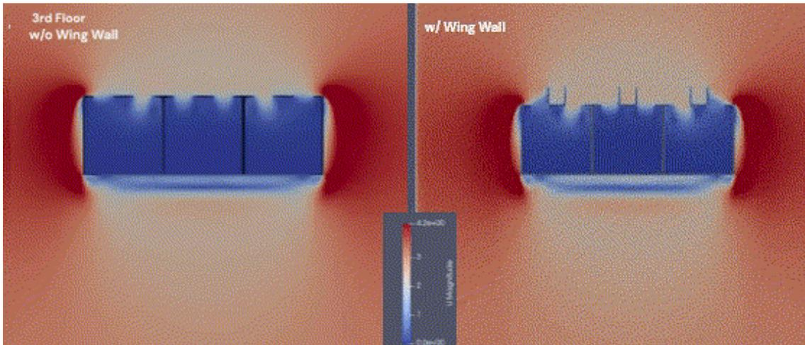
Figure 17. Velocity distribution at the third floor without wing wall (left) and with wing wall (right).
