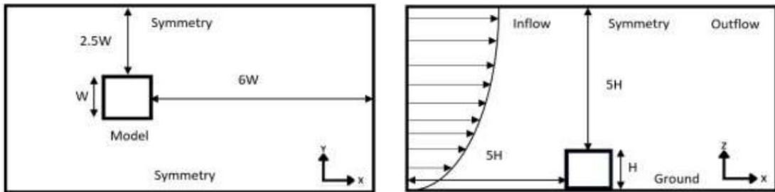
Figure 12. Computational domain and boundary conditions for the simulation, showing inflow, outflow, ground, and symmetry planes relative to the building model.
