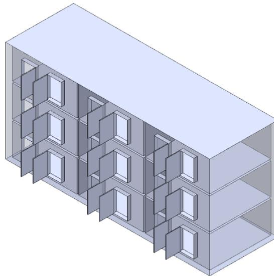
*Figure 1. Multi-unit multi-storey building with wing walls.*
